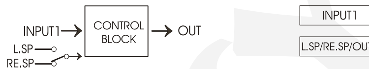
Fig. 24 - Diagram of control blocks and display for remote setpoint
